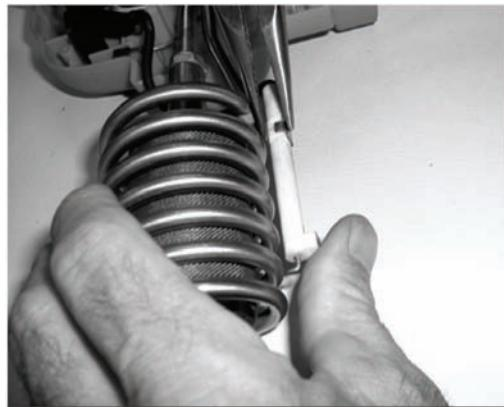
7. NOTE: Be sure pump rod is attached to pump handle.
