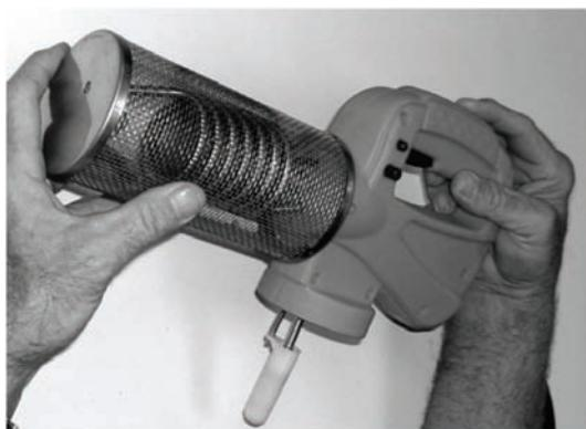
9. Place upper housing over assembly unit until halves line up and ignitor works. Replace 6 screws.
