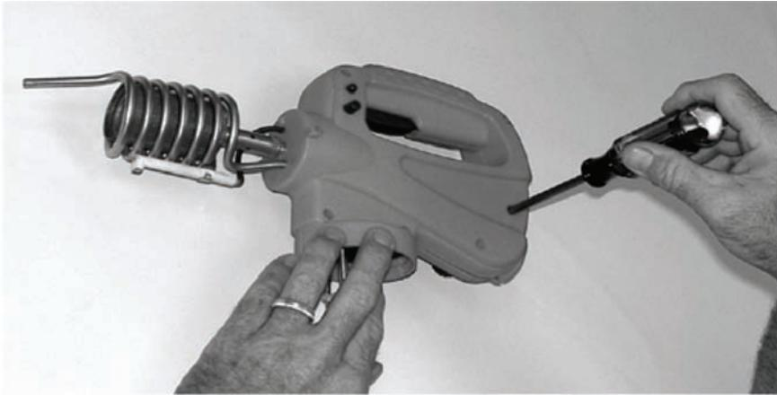
4. Remove upper half of housing to reveal inside of fogger.
