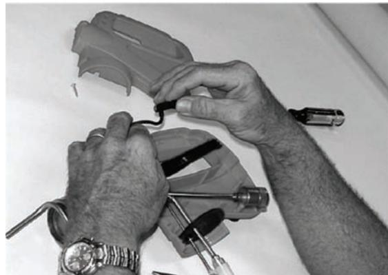
6. Lift out old ignitor and replace with new ignitor. Ignitor tip should be within 1/8 inch of coils. Retighten crimp while holding ignitor firmly in place.
