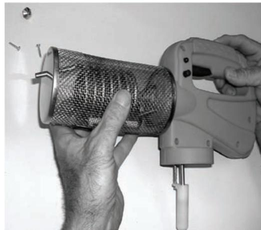
2. Remove Coil wire basket. Some gentle tapping may be required on the end of the fluid distribution tube.
