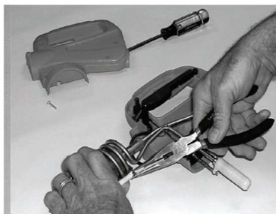
5. Using needle nose pliers, open ignitor crimp while holding structure firmly in place.
